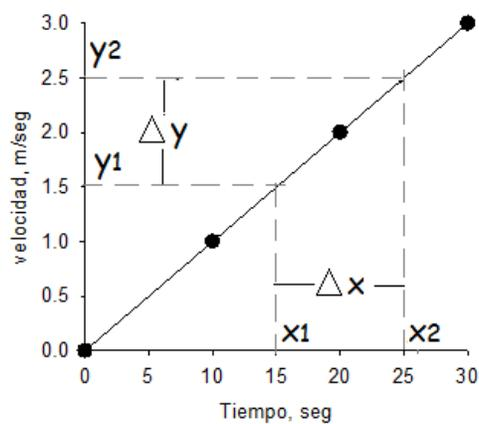
$$a = \frac{\Delta y}{\Delta x} = \frac{v_2 - v_1}{t_2 - t_1} = \frac{(2,5 - 1,5) \text{ m/s}}{(25 - 15) \text{ s}} = 0,1 \frac{\text{m}}{\text{s}^2}$$
