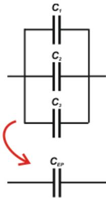
$$C_{EP} = C_1 + C_2 + C_3 + \dots + C_n$$
