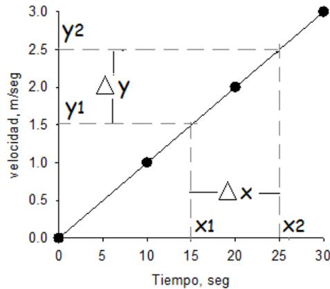
$$a = \frac{\Delta y}{\Delta x} = \frac{v_2 - v_1}{t_2 - t_1} = \frac{(2,5 - 1,5)m/s}{(25 - 15)s} = 0,1 \frac{m}{s^2}$$
