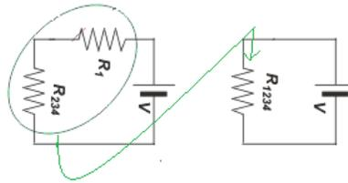
$$R_{1234} = R_1 + R_{234}$$
